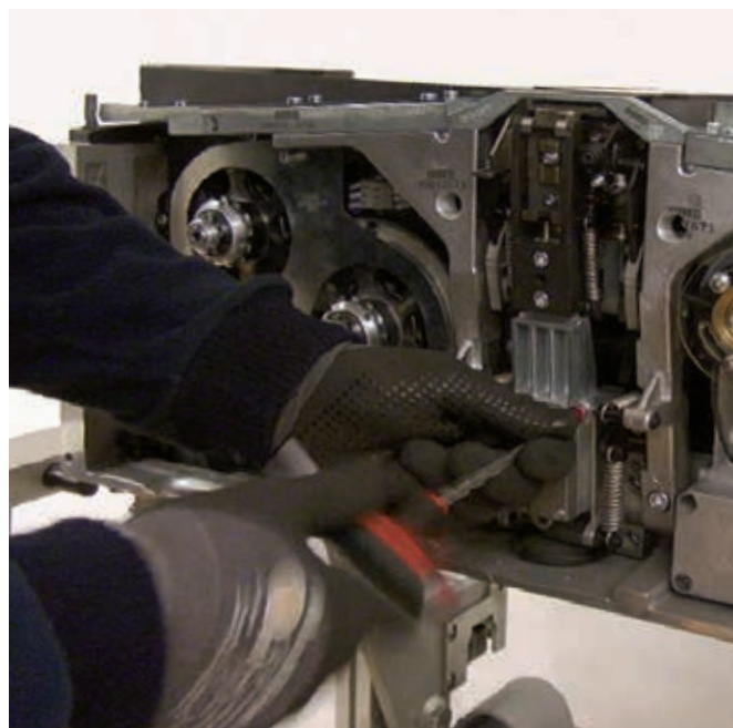
Detail of fast replacement of Welding Group.
