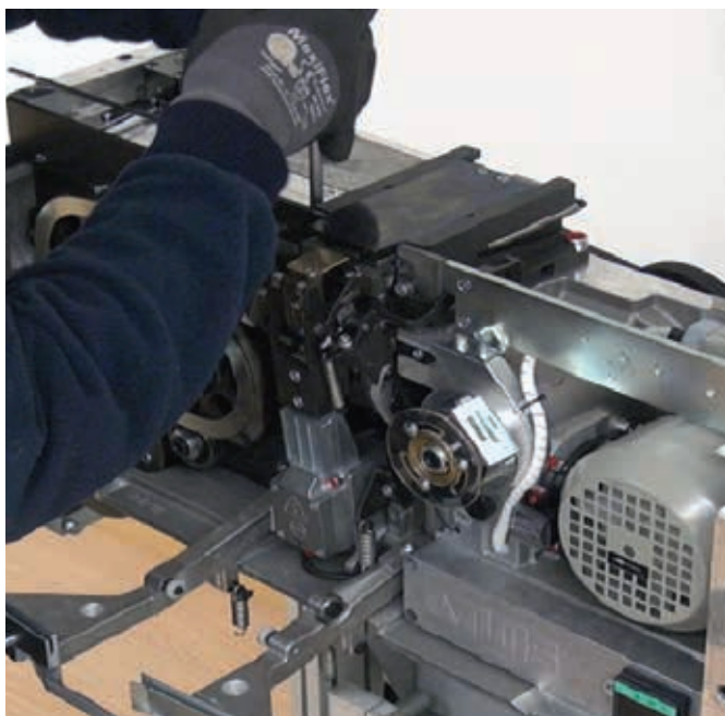
Detail of fast replacement of Clamping Group.
